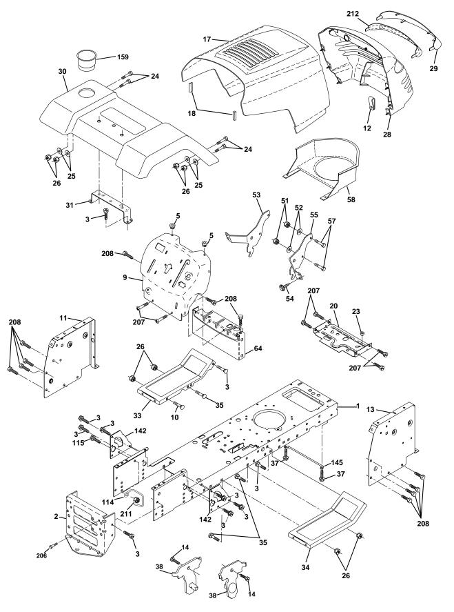
TRACTOR - - MODEL NUMBER PR18542STC CHASSIS AND ENCLOSURES
